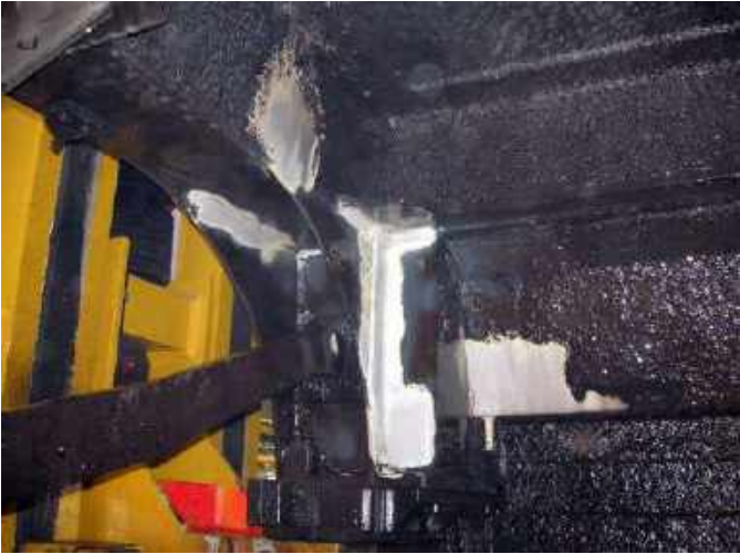
Removal of corrosion protection on a train for weld inspection
